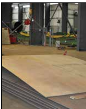
PLATE The raw material – pieces of flat steel plate – is received into our manufacturing plant.
