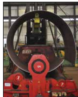
BENDING After beveling, the plate is transferred to the bending rolls. Nucor Skyline uses a 4-roll system to produce a true cylinder, also referred to as a can.
