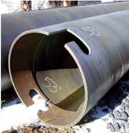
Pipe with Slots
