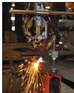
BEVELING After the plate is cut, it is transferred to the beveling station where different bevel angles are cut into the plate edge for welding.
