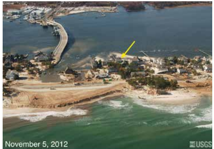
Oblique aerial photographs of Mantoloking, NJ. View looking west along the New Jersey shore. Storm waves and surge cut across the barrier island at Mantoloking, NJ, eroding a wide beach, destroying houses and roads, and depositing sand onto the island and into the back-bay. Construction crews with heavy machinery are seen clearing sand from roads and pushing sand seaward to build a wider beach and protective berm just days after the storm. The yellow arrow in each image points to the same feature. (PHOTO: USGS)
