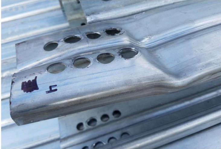
Figure 3-2: Cantilever Testing Failure
