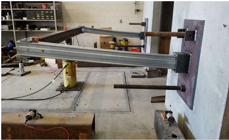
Figure 3-1: Cantilever Testing Configuration
