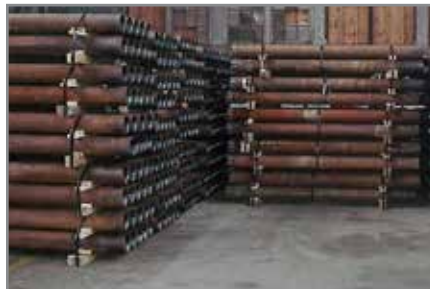
Female and male casing cut and bundled to specifications
